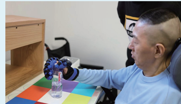
Fig. 2 The patient grasps a bottle using the NEO wireless BCI system and a prosthetic hand. Electrodes were implanted over his primary sensory and motor cortex (S1 and M1) to collect ECoG signals above the dura matter, while he attempted to grasp the bottle.
